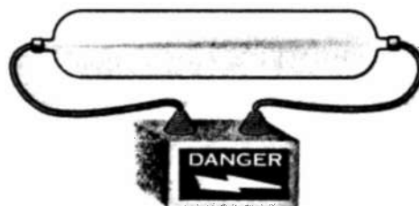
high voltage electricity creating cathode rays inside a Crookes tube
