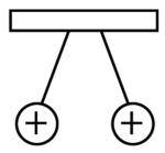
An object is neutral and has no charge when it has the same amount of protons and electrons. But when the object loses or gains electrons it becomes unbalanced, and electrically charged. If there are more protons than electrons, the object carries a positive charge. If there are more electrons than protons, the object carries a negative charge.
