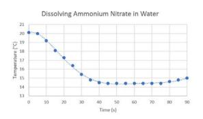
16. A student designed an experiment to measure the heat of solution for ammonium nitrate – a common ingredient in cold packs. She added solid NH<sub>4</sub>NO<sub>3</sub> to water in a coffee cup calorimeter that was placed on a magnetic stirrer to mix the contents. She used a sensor to measure the temperature change and obtained the graph shown above.
