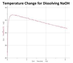
13. A student did a calorimetry experiment to determine the **enthalpy of dissolution** for sodium hydroxide. She used a sensor to measure the temperature change in a **calorimeter** while dissolving a sample of NaOH in distilled water. Use her data below and the graph above to find  $\Delta H_{solution}$  for NaOH, expressed as "kJ/mol rxn".
