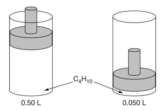
A sample of  $C_4H_{10}(g)$  is placed in a rigid vessel with a movable piston. The volume of the gas is reduced by moving the piston downward while the temperature is maintained at  $25\,^{\circ}$ C, as shown above. The pressure of the gas versus its volume is plotted in the graph below.
