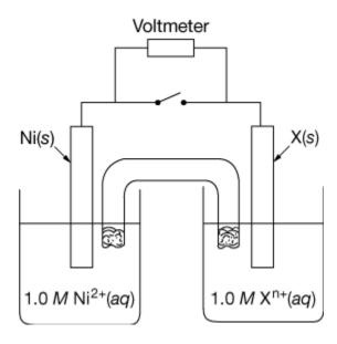
In the galvanic cell shown above, the voltmeter connected across the electrodes shows a voltage of  $0.52\ V$ . Based on the standard reduction potentials given in the table below, which of the following is most likely the identity of the unknown element, X?
