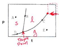
Label the "triple point" on the diagram. Label the "critical point" on the diagram.
