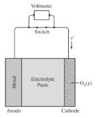
Metal-air cells are a relatively new type of portable energy source consisting of a metal anode, an alkaline electrolyte paste that contains water, and a porous cathode membrane that lets in oxygen from the air. A schematic of the cell is shown above. Reduction potentials for the cathode and three possible metal anodes are given in the table below.
