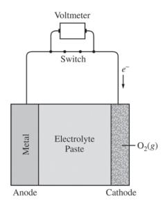
2. Metal-air cells are a relatively new type of portable energy source consisting of a metal anode, an alkaline electrolyte paste that contains water, and a porous cathode membrane that lets in oxygen from the air. A schematic of the cell is shown above. Reduction potentials for the cathode and three possible metal anodes are given in the table below.
