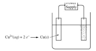
3. An external direct-current power supply is connected to two platinum electrodes immersed in a beaker containing 1.0 M CuSO<sub>4</sub>(aq) at 25°C, as shown in the diagram above. As the cell operates, copper metal is deposited onto one electrode and O<sub>2</sub>(g) is produced at the other electrode. The two reduction half-reactions for the overall reaction that occurs in the cell are shown in the table below.
