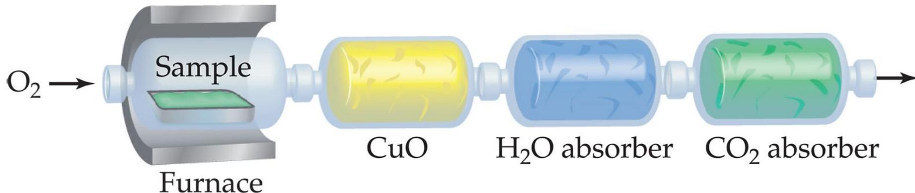
**Compounds containing C, H and O are routinely analyzed through combustion in a chamber like this.**
