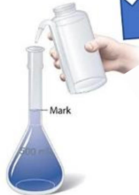
(d) Additional solvent is added up to the mark on the volumetric flask.
